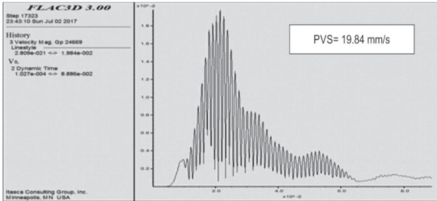
Fig.6 Simulation result of blast vibration recorded at 50m radial distance for blasthole of diameter 100mm and depth 20m with 14m charge column length
