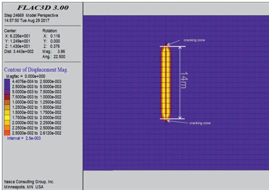
Fig.11 Contour of displacement magnitude for 20m blasthole depth with 14m charge length
