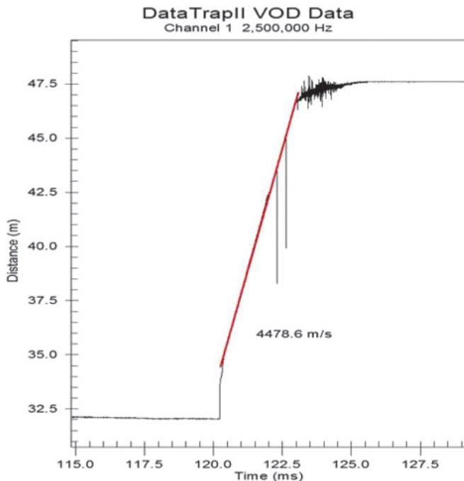
Fig.5 Plot of recorded VOD of ANFO explosive for 311mm diameter blasthole at dragline bench
