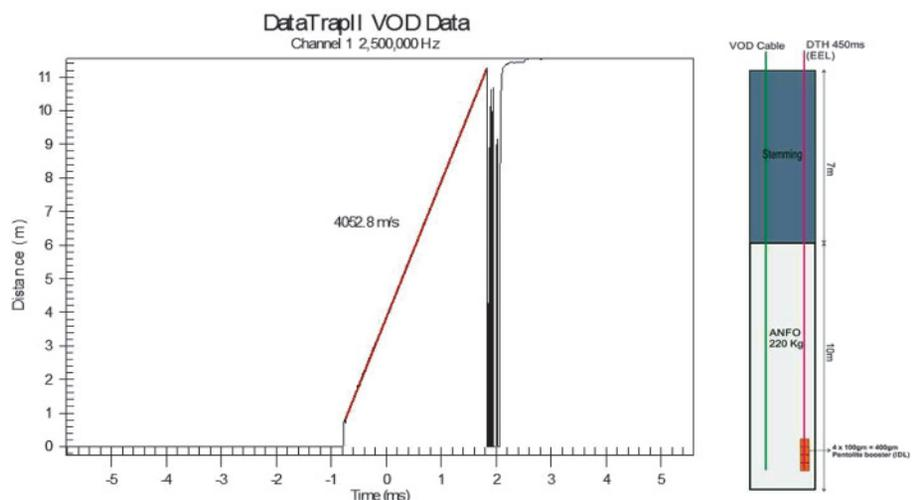
Fig.4 Plot of recorded VOD of ANFO explosive for 159mm diameter blasthole at shovel bench
