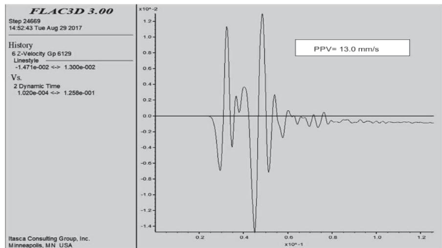
Fig.10 Vertical directional vibration resulted from simulation of blasthole of depth 20m with charge length 14m at radial distance of 50m and vertical distance of 17m
