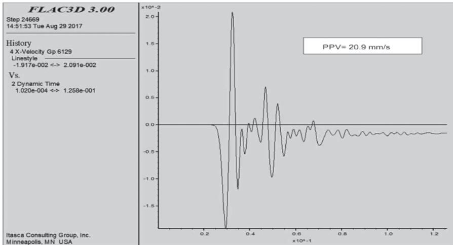
Fig.8 Longitudinal vibration resulted from simulation of blasthole of depth 20m with charge length 14m at radial distance of 50m and longitudinal distance of 43m
