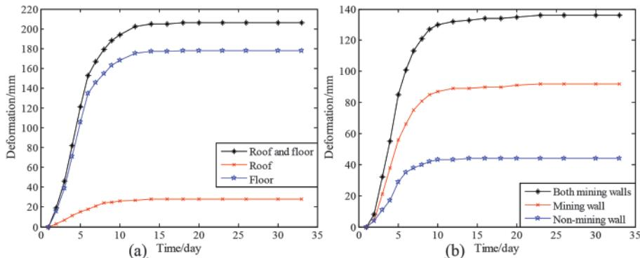
Fig.7 Deformation of roadway surrounding rock with combined support
