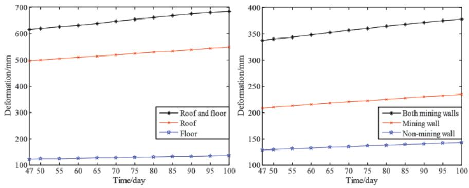
(a) Displacement of roof and floor of roadway (b) Displacement of both sides of roadway
