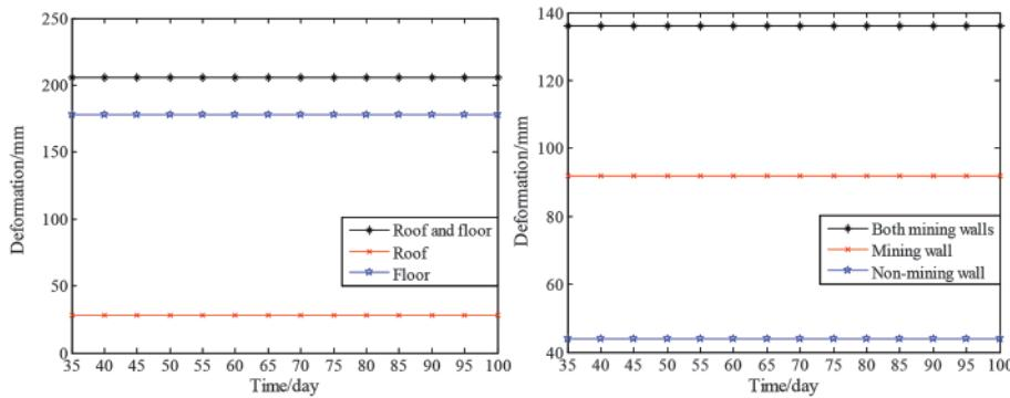
(a) Displacement of the roadway roof and floor (b) Displacement of both roadway sides
