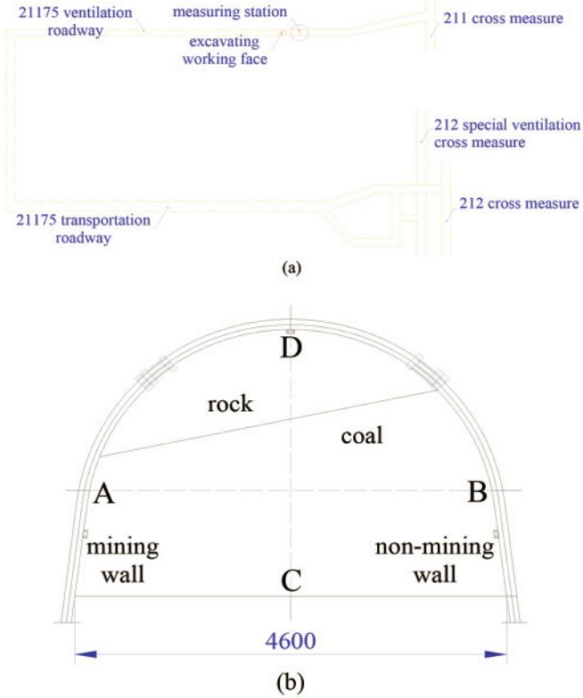
Fig.3 Layout of the monitoring station of surrounding rock deformation
