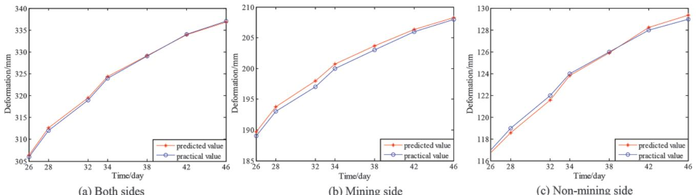
Fig.5 Displacement of both sides of roadway
