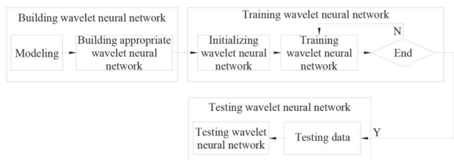
Fig.2 Training process of the wavelet neural network
