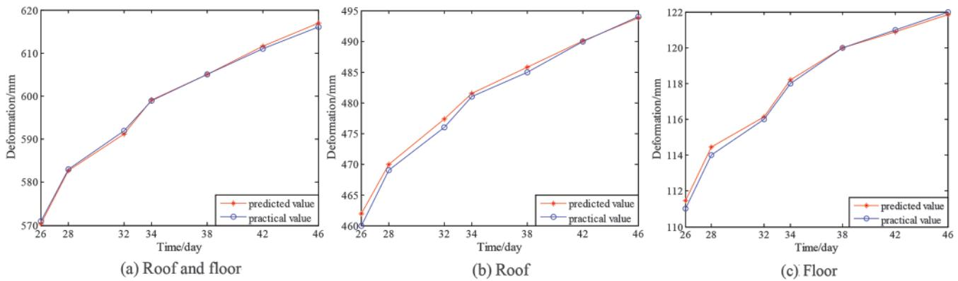
Fig.4 Displacement of roof and floor of roadway
