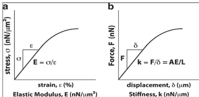
Figure 5: Definitions of (a) the elastic modulus, (b) stiffness
