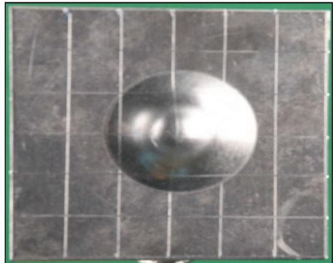
Figure 2: Al sheet metal with 10 x 10 mm square pattern
