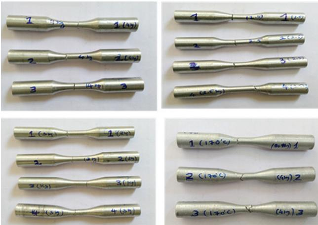
Fig.2. Fractured fatigue specimen's
