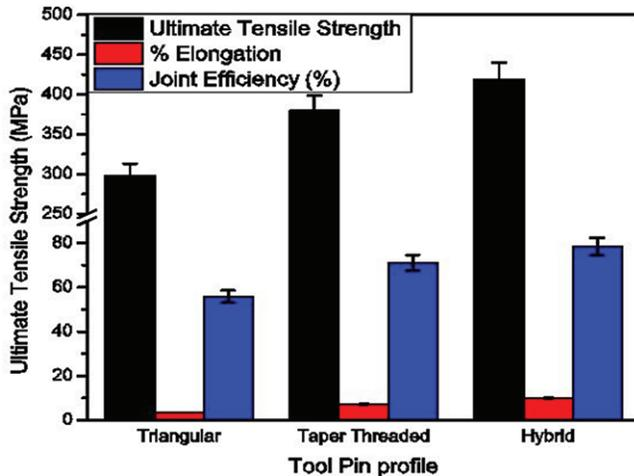
Fig.4: The tensile properties of the joints by using the different tool pin profile
