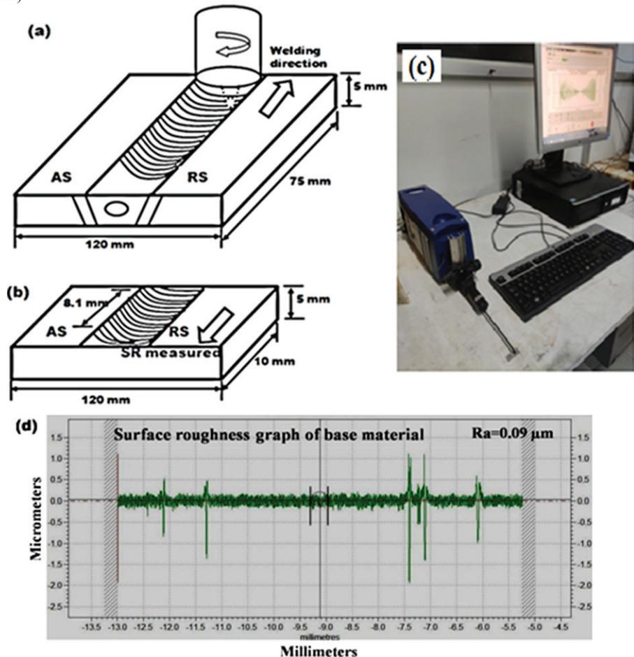
Fig.2: (a) Friction stir welded specimen (b) direction of measurement of surface roughness (c) set up of surface roughness tester machine (d) roughness of the base material.
