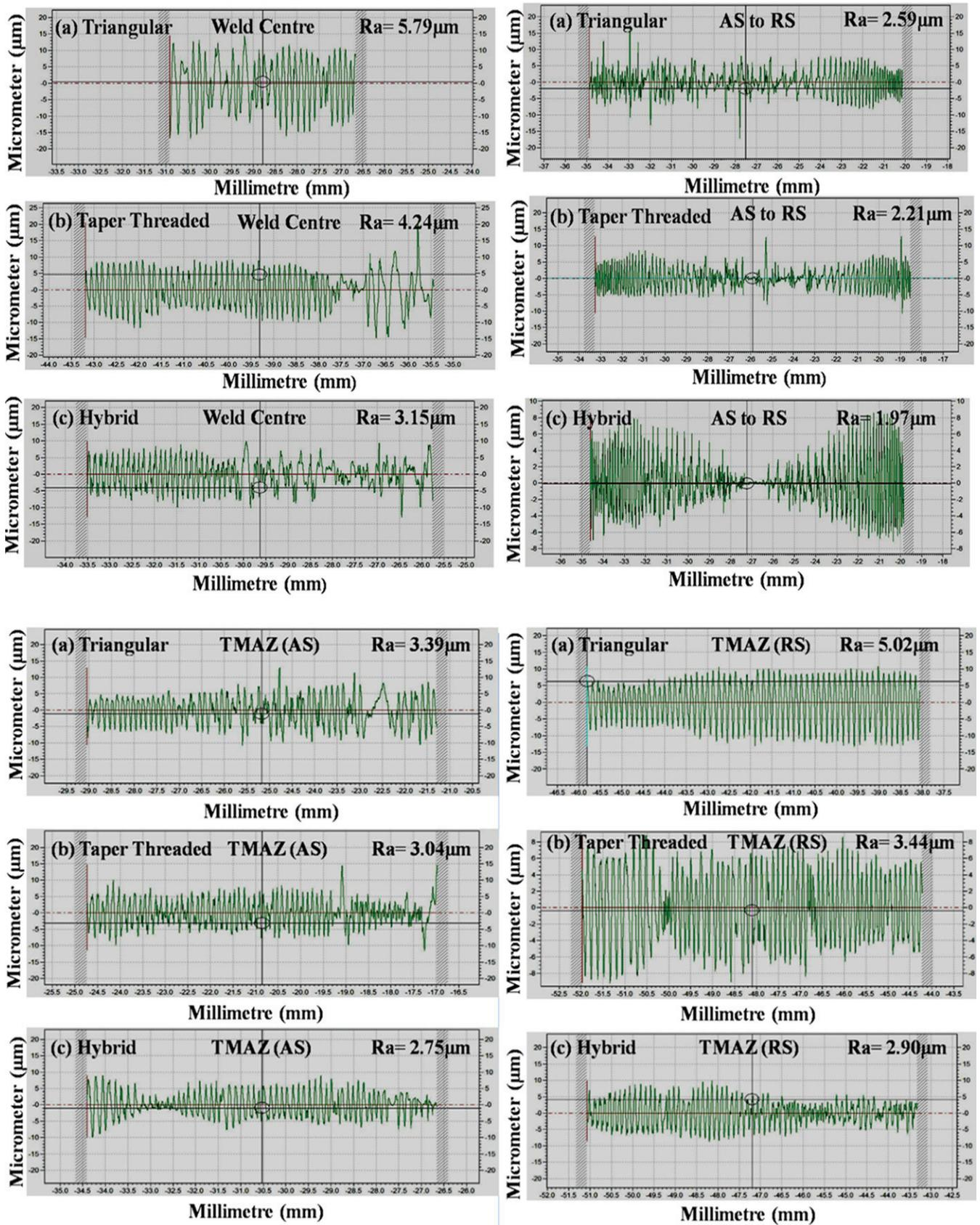
Fig.3: Surface roughness graph of friction stir welded samples using different tool geometry (a) Triangular, (b) Taper threaded and (c) Hybrid at the different portion of welded samples (weld centre, AS and RS of TMAZ and AS to RS)
