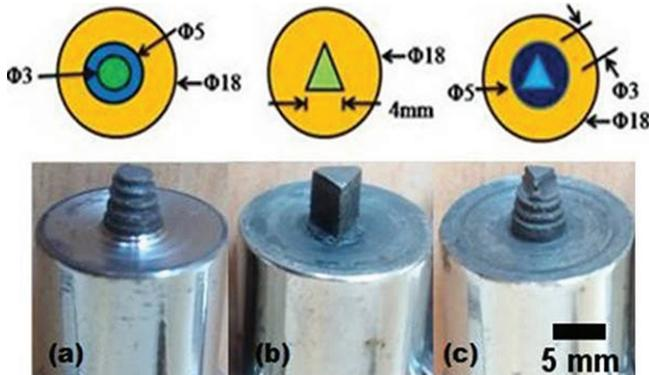
Fig.1.: Different friction stir tools were used for the experiment; (a) a taper threaded tool (b) a triangular tool and (c) The hybrid tool pin (HTP)
