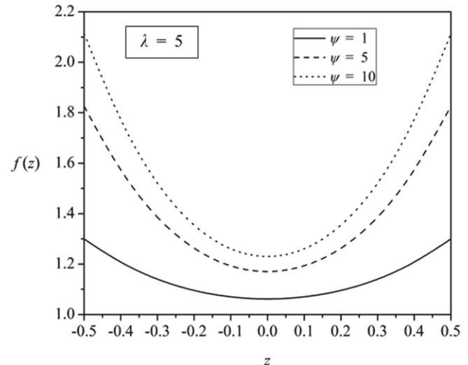
Fig.1: Basic temperature profiles for different values of the conduction-radiation parameter  $\psi$ .
