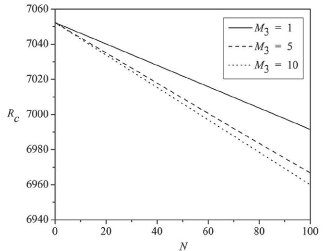
Fig.7: Plot of  $R_c$  as a function of  $N$  for different values of  $M_3$  and  $Da^{-1}=5, \Lambda=3, \psi=5, \lambda=5, \chi=2$ .
