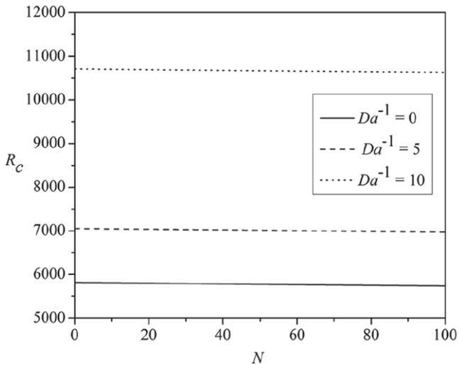
Fig.4: Plot of  $R_c$  as a function of  $N$  for different values of  $Da^{-1}$  and  $\Lambda=3, \psi=5, \lambda=5, M_3=3, \chi=2$ .
