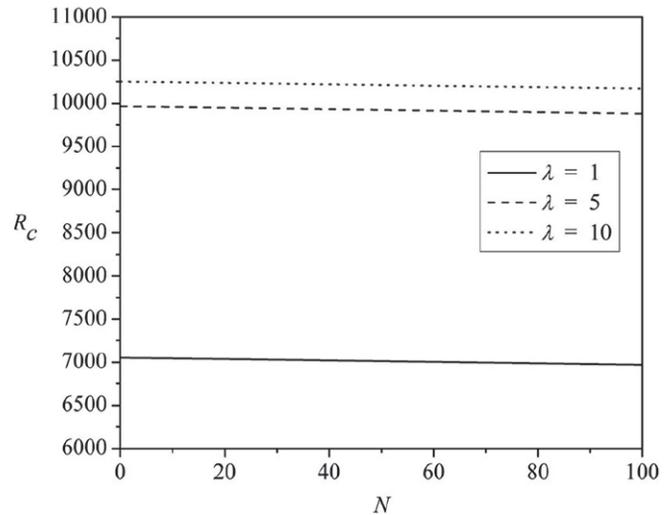
Fig.6: Plot of  $R_c$  as a function of  $N$  for different values of  $\lambda$  and  $Da^{-1}=5, \Lambda=3, \psi=5, M_3=3, \chi=2$ .
