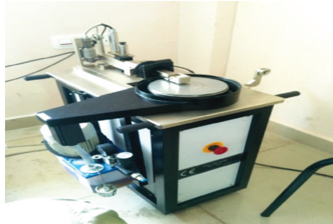
Fig.1: Pin-on-disc wear testing apparatus
