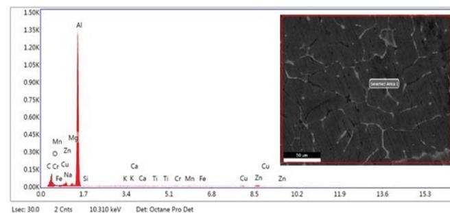
Fig.3: EDS spectrum analysis of Al7075 6 wt. % Beryl-2 wt. % GNPs hybrid composites
