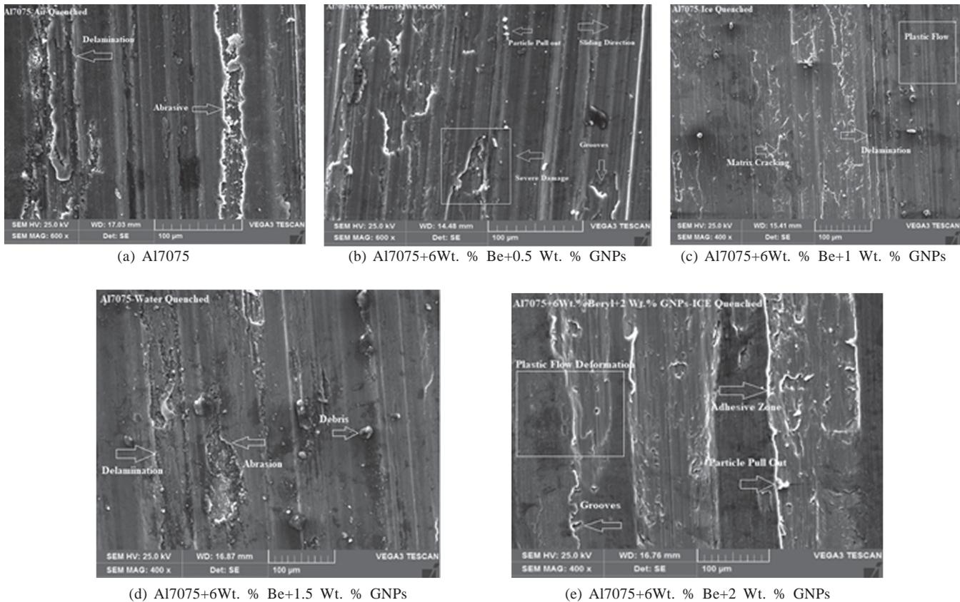
Fig.9: SEM results worn surfaces of heat-treated ice quench at different loads
