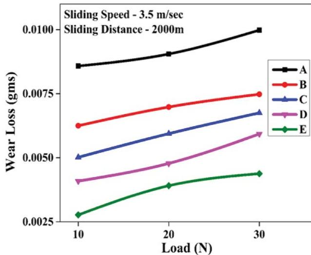
Fig.6: Wear loss of as-cast Al7075 and its hybrid composites at different loads
