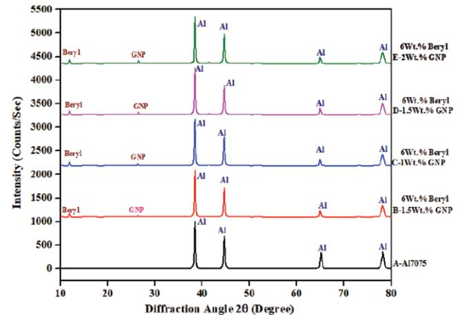
Fig.5: X-Ray diffraction patterns of Al7075 and its composites
