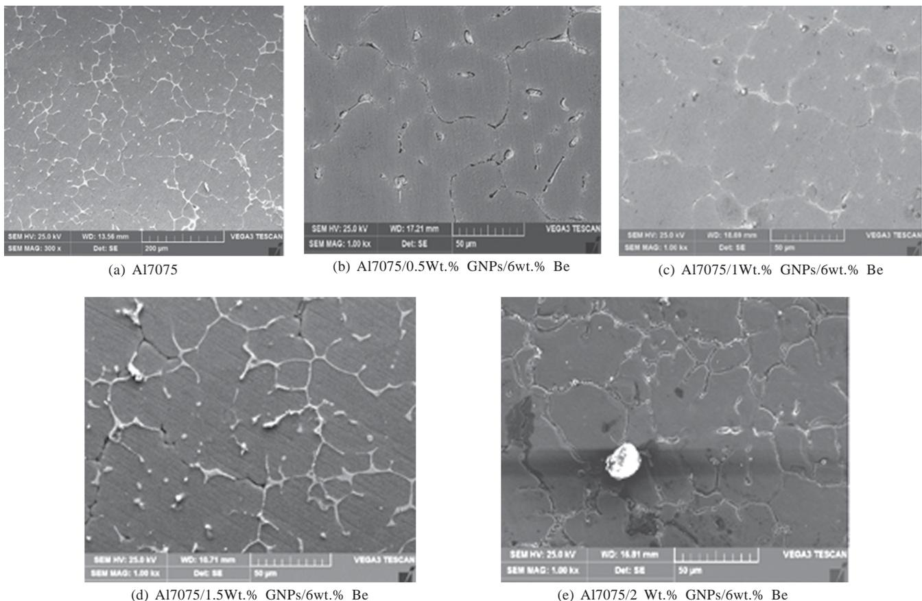
Fig.1: SEM image of Al7075 and its hybrid composites
