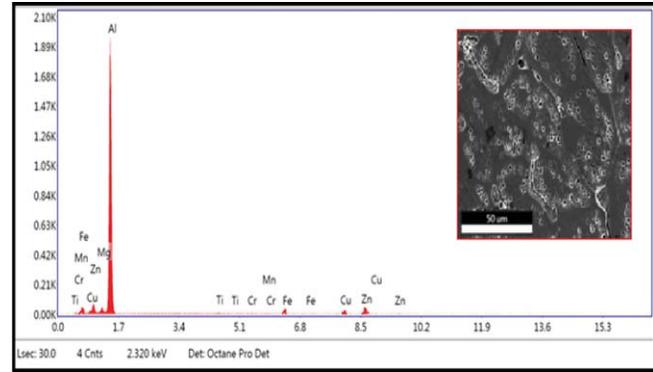
Fig.4: EDS of T6 ice quench Al7075 matrix
