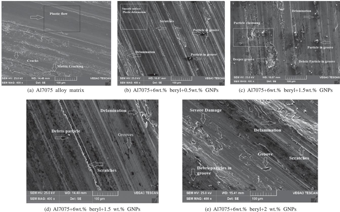
Fig.8: SEM results of worn surfaces at load 30N, sliding distance 2000m, and sliding speed 3.5m/sec
