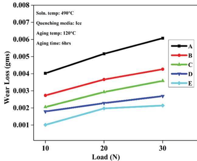
Fig.7: Variation of wear loss of heat-treated ice quenched Al7075 and its hybrid composites at different loads
