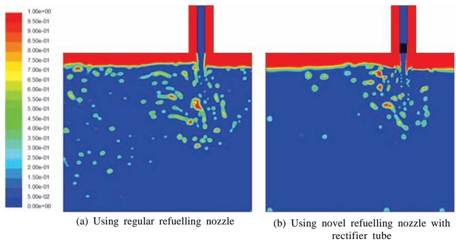
Fig.5. Contours of oil and gas volume fraction at  $t=13.5s$
