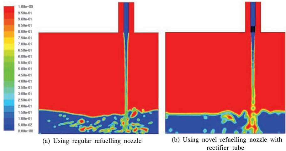
Fig.3. Contours of oil and gas volume fraction at  $t=3s$
