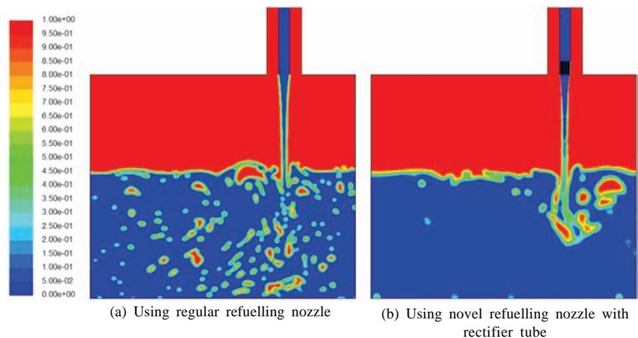
Fig.4. Contours of oil and gas volume fraction at  $t=8s$
