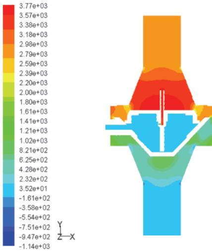
Fig.6 Pressure contours of  $Z = 0$  plane
