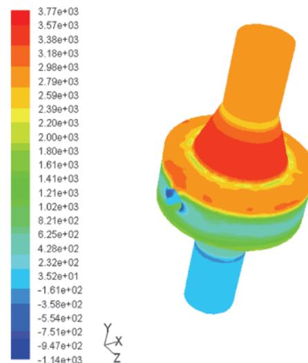
Fig.5 Pressure contours of exterior surface
