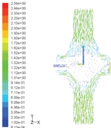
Fig.9 Velocity vectors of  $Z = 0$  plane
