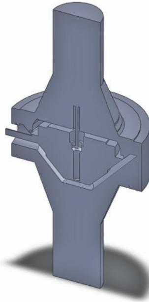
Fig.1 Geometric model of control valve internal flow field (cross-section drawn)
