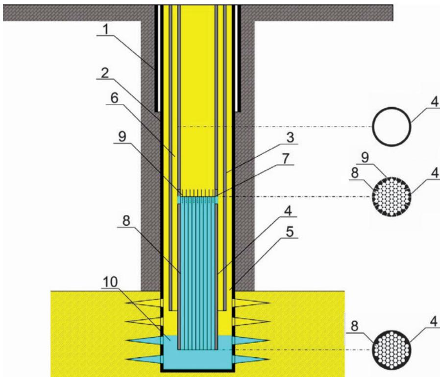
Fig.5 The conceptual model of fluid recovery from the bottom-hole
