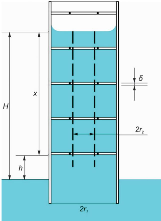
Fig.4 The capillary with perforation holes
