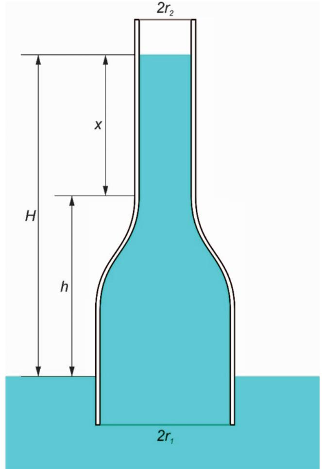
Fig.3 The capillary tube with an uneven cross-sectional radius
