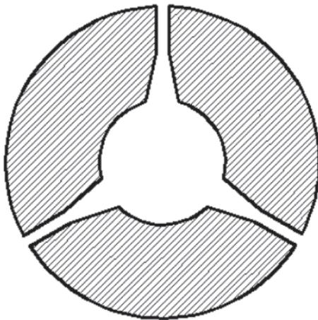
Fig.7 Profile of drill pipe
