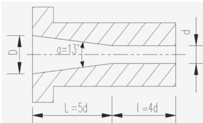
Fig.1 Schematic picture of nozzle
