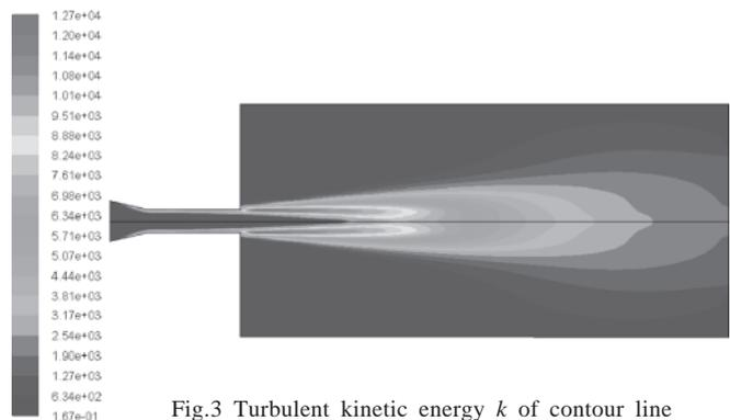
Fig.3 Turbulent kinetic energy  $k$  of contour line
