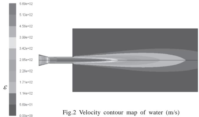
Fig.2 Velocity contour map of water (m/s)
