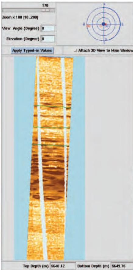
Fig.12a Both the apparent and true dip of chert nodule and chert banding distributed along the formation are very low in vertical well (well A12)
