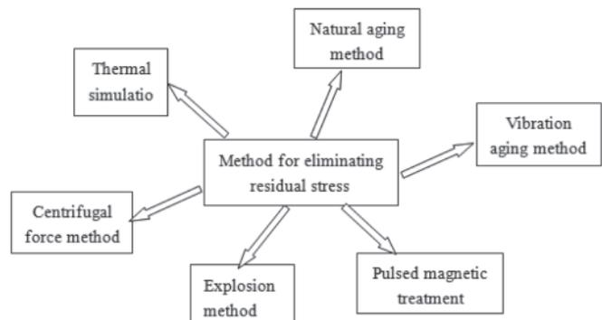
Fig.3 Residual stress relief methods
