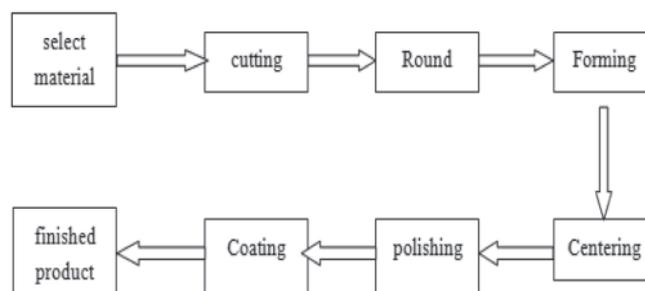
Fig.1 Traditional aspheric mirror processing flow
