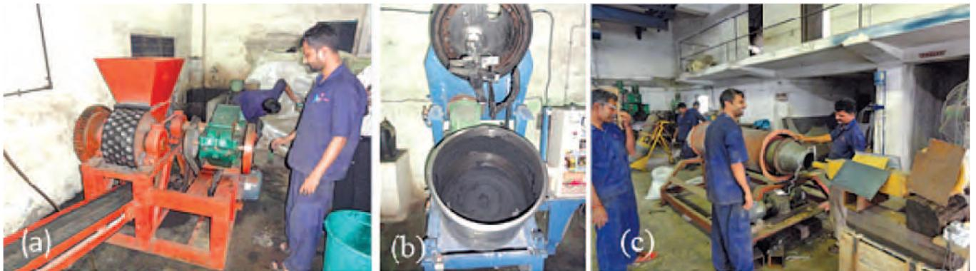
Fig.2 Laboratory equipment (a) Coal crusher (b) Vessel (c) Rotary drier
