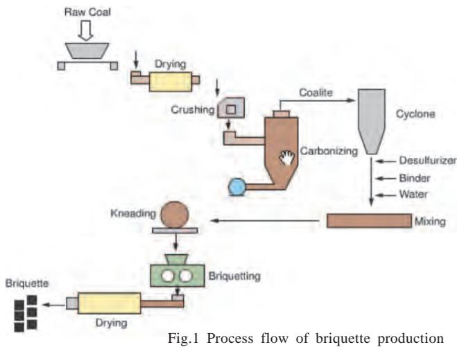
Fig.1 Process flow of briquette production
