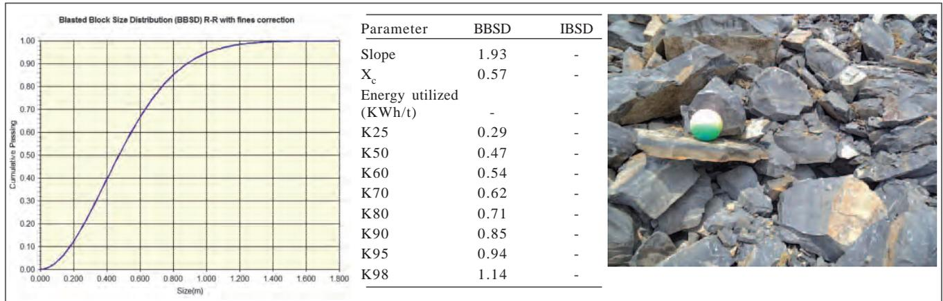
Fig.4 Digital image analysis for measuring the fragmentation in the limestone quarry
