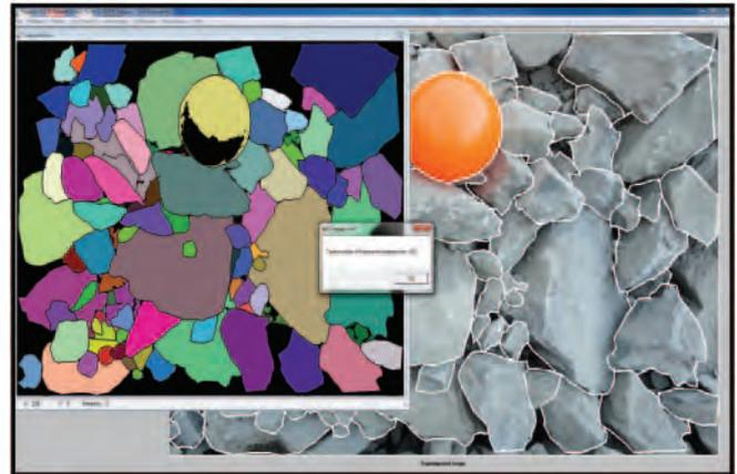
Fig.2 Fragmentation analysis using Fragalyst image analysis software
