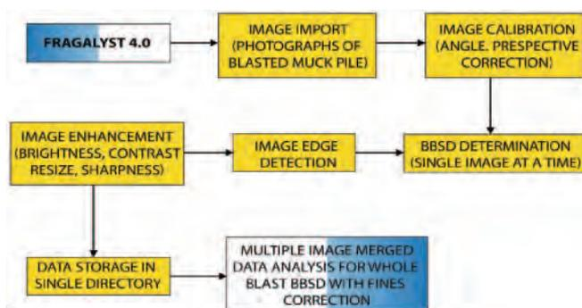
Fig.1. Different steps involved in analysing the image of a blast muckpile
