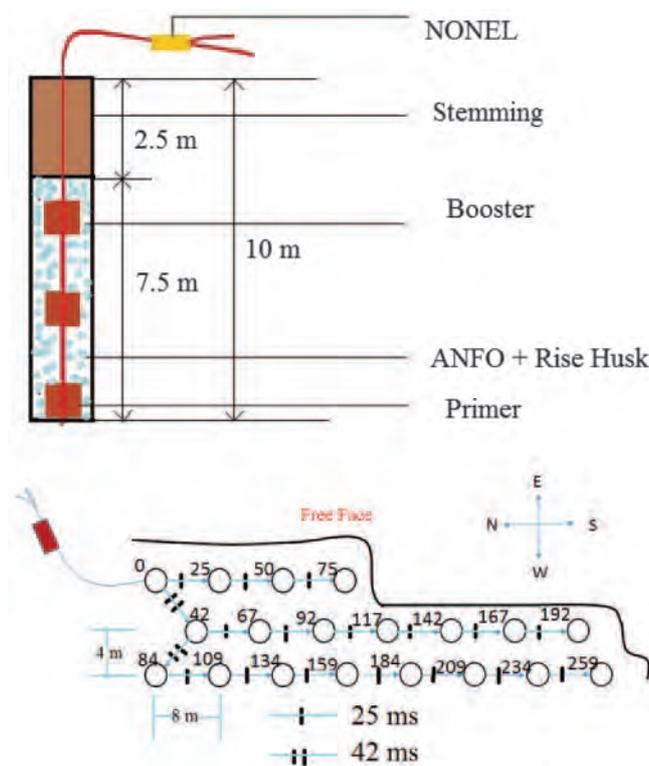
Fig.3 Charging and initiation pattern for a blast in the limestone quarry
