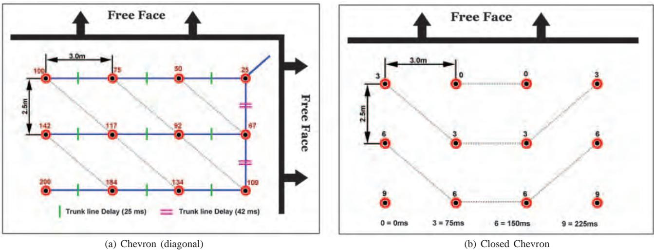
Fig.5 Schematic representation of the Initiation patterns used in the blasts carried out in the aggregate stone quarry
