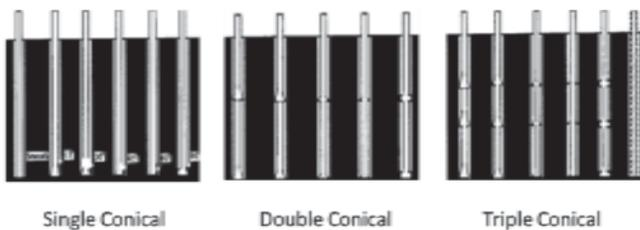
Fig.6 Different type of bolt used in the test
