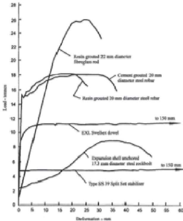
Fig.5 Load-deformation results obtained by Stillborg (1994) in tests carried out at Lulea University in Sweden
