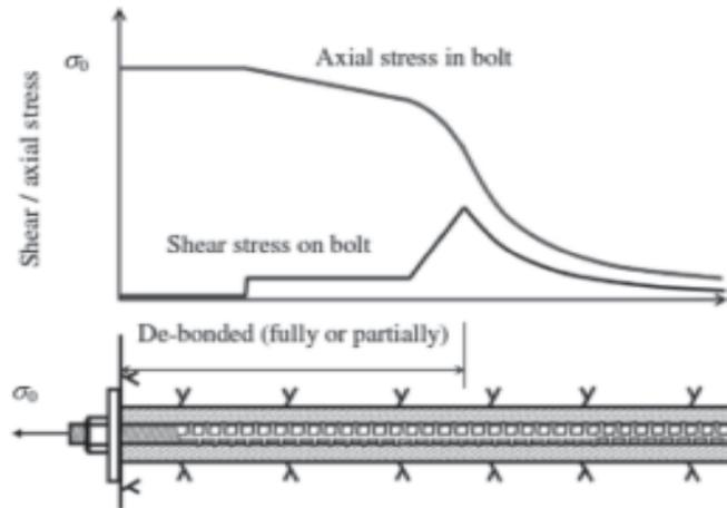
Fig.3 Stress distribution along the bolt length in pull-out test (Li et al., 2014)
