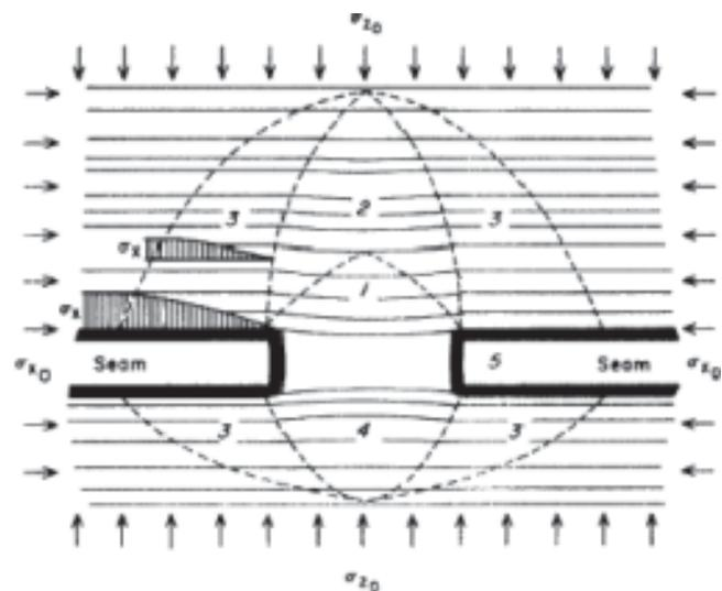
Fig.2 Stress distribution around an opening (Peng, 1986)
