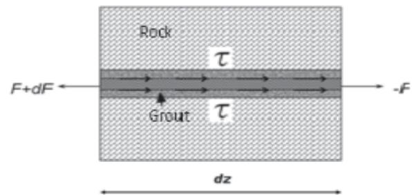
Fig.4 Load transfer and stress distribution in fully grouted rock bolt (Singh et al., 2016a)
