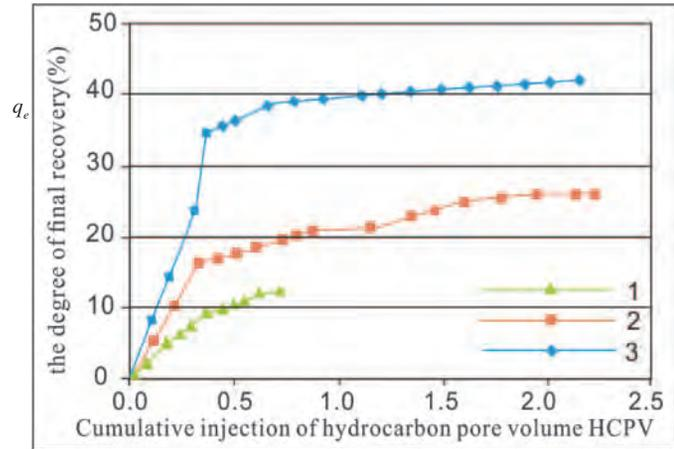
Fig.7 Water injection production curve of tight tuff oil cores with different wettabilities
