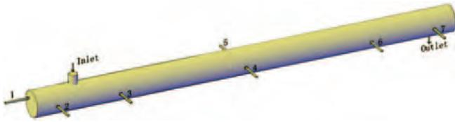
Fig.2 Distribution of the points for vibration measurement
