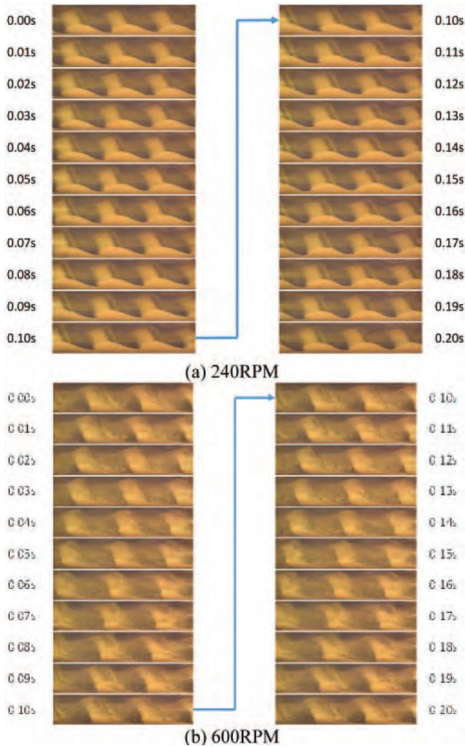
Fig.8 Dynamic comparison from the back for over 0.2s. The shooting frame rate is 500 frames per second, and the 21 frames in (a) and (b) are evenly selected from 100 frames in 0.2s
