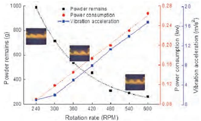
Fig.10 Comparison between curves of powder residue, power consumption and vibration acceleration
