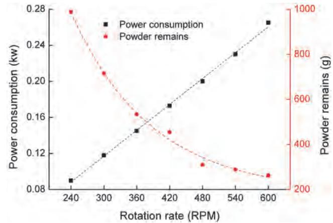
Fig.4 Comparison of power consumption curve and powder transport curve
