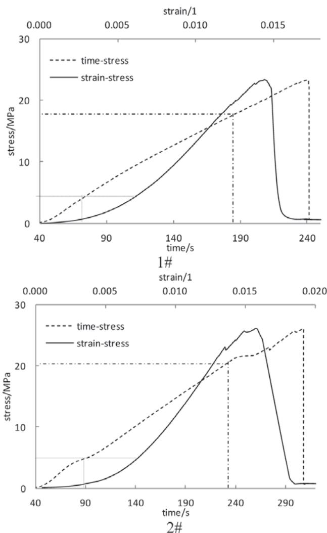
Fig.4 Stress-strain-time graphs of coal samples
