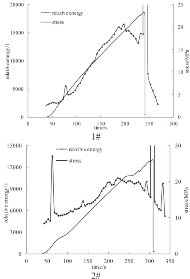
Fig.5 Variation diagrams for relative energy of infrasonic waves over the loading time
