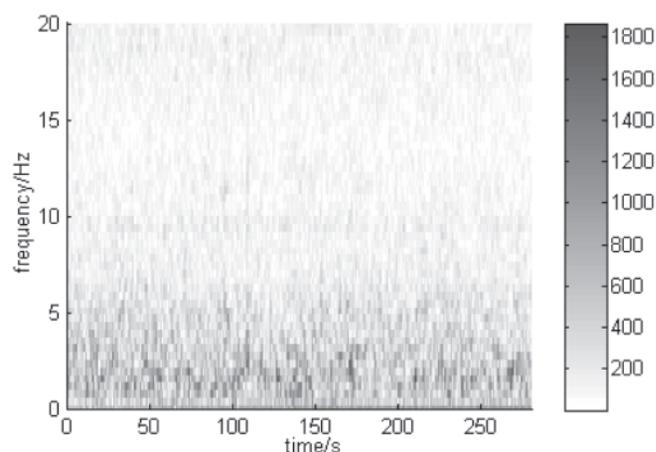
Fig.3 Test results of ambient noise (the grayscale represents the intensity)
