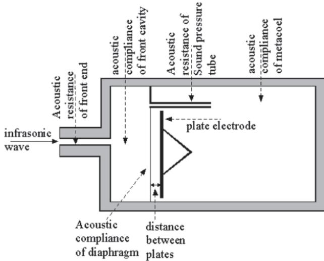
Fig.2 Work principle diagram of CASI-ISM-2013 infrasound sensor
