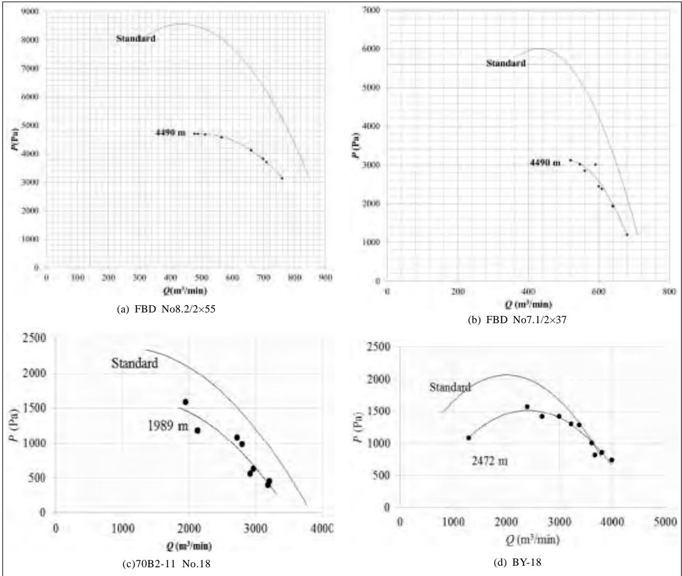
Fig.1 Contrast of the P-Q characteristic curves of fans at different altitudes
