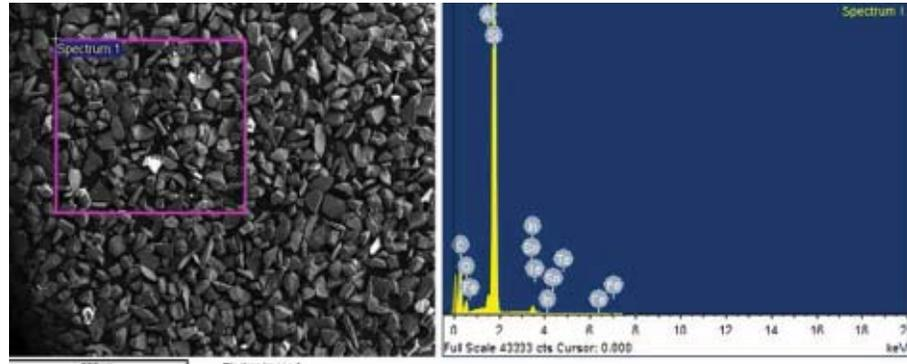
Fig.1 : SEM image of fly ash particles
