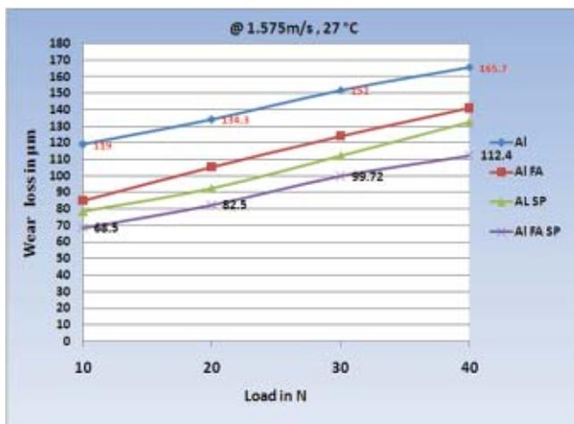
Fig.6 Wear loss of composites with respect to load, sliding velocity of 1.575 m/s at 27°C
