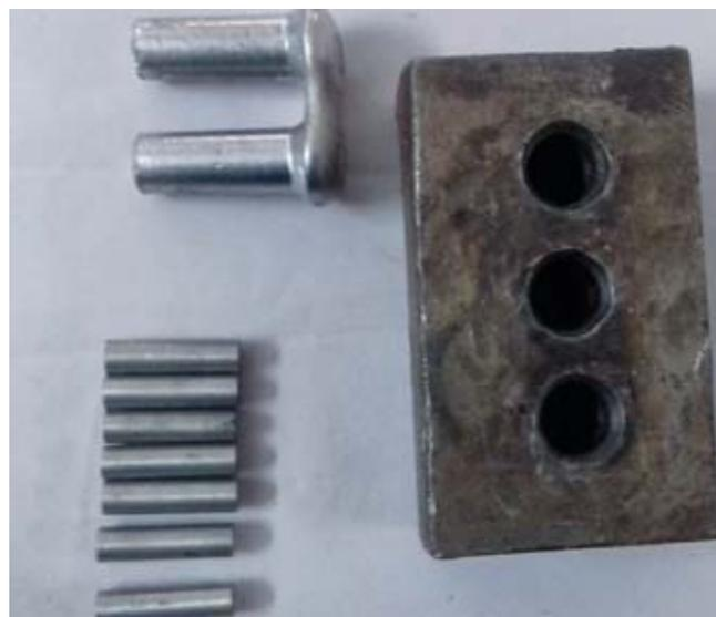
Fig.5 Wear pins with die
