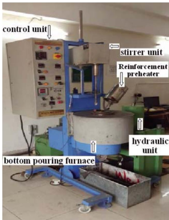
Fig.3 Modified squeeze casting set up
