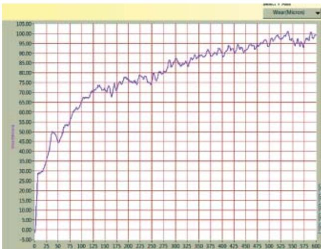
Fig.10 Wear loss of composites with respect to load, sliding velocity of 3.142 m/s at 90°C
