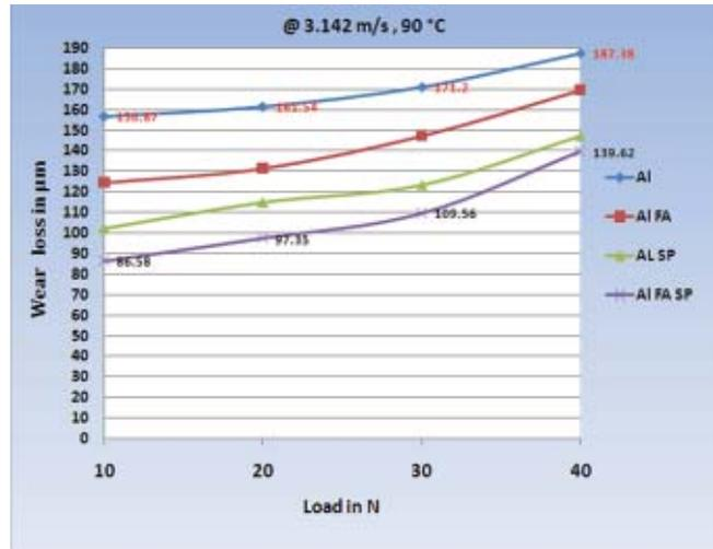
Fig.11 Wear loss of Al/FA/SP hybrid composite with respect to load of 40N, velocity of 3.142 m/s at 27°C
