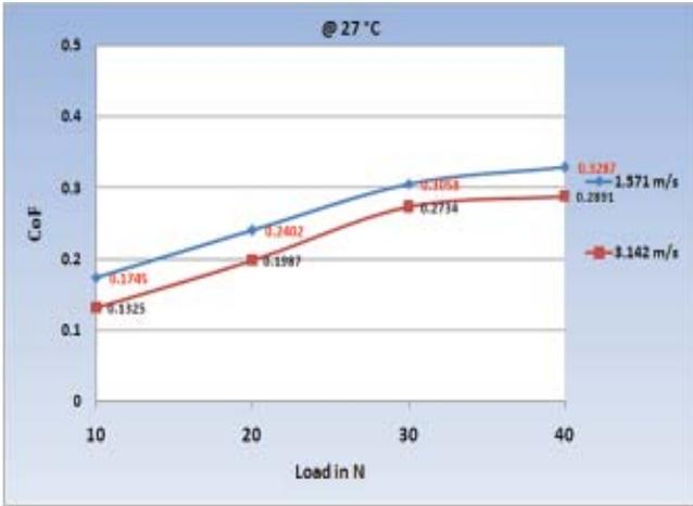
Fig.12 Co-efficient of friction of LM25/FA/SP hybrid composites as a function of load, sliding velocity at 27°C
