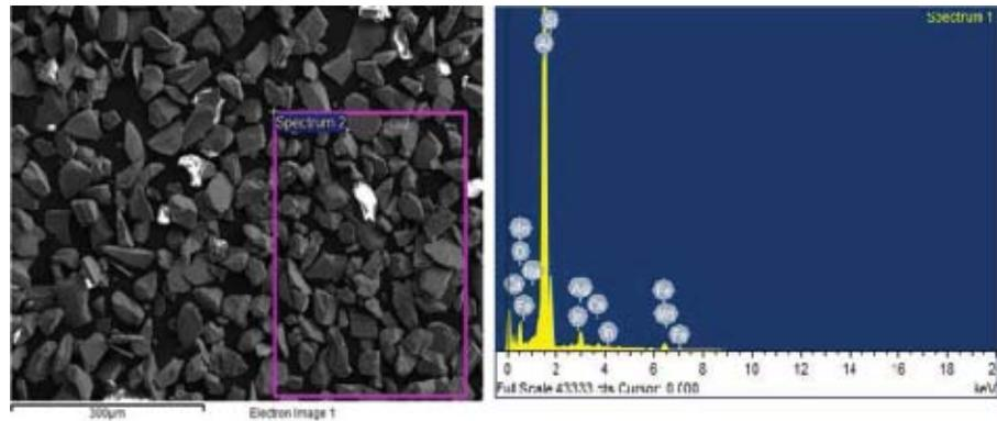
Fig.2 SEM image of steel particles
