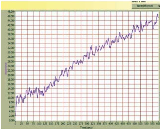
Fig.9 Wear loss of Al/FA/SP hybrid composite with respect to load of 10N, velocity of 3.142 m/s at 27°C.
