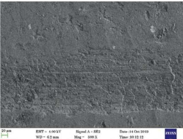
Fig.14 SEM image of the worn surface of the Al LM25 (normal load of 40N, 1.571 m/s sliding velocity at a pin temperature of 27°C)
