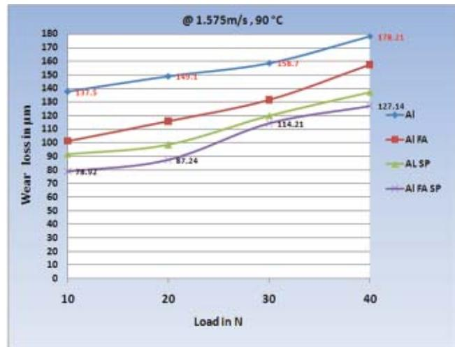
Fig.7 Wear loss of composites with respect to load, sliding velocity of 1.575 m/s at 90°C
