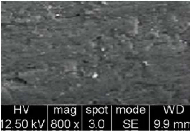
Fig.17 SEM image of the worn surface of the Al LM25/FA/SP hybrid composite (normal load of 40N, 1.571 m/s sliding velocity at a pin temperature of 90°C)
