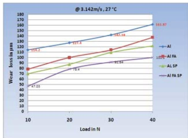
Fig.8 Wear loss of composites with respect to load, sliding velocity of 3.142 m/s at 27°C
