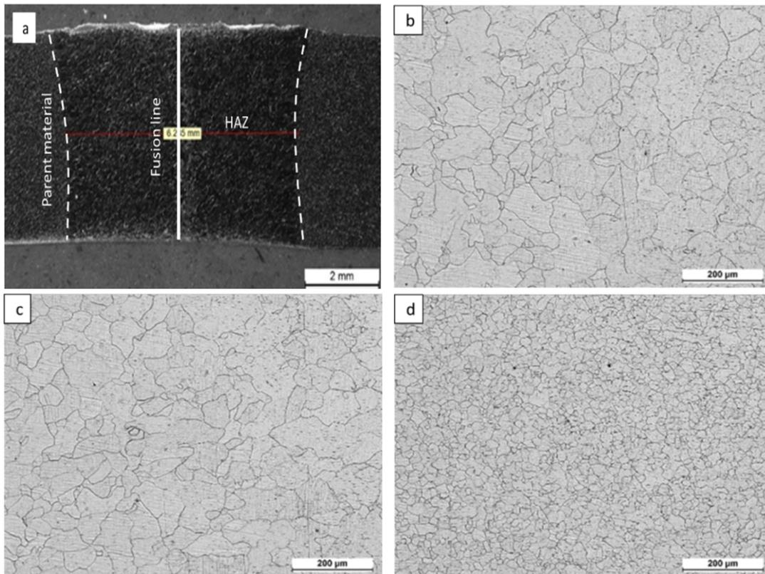
Fig. 2 : Optical image of a) Stereo of FB weld, b) Fusion line, c) Heat affected zone, and d) parent material
