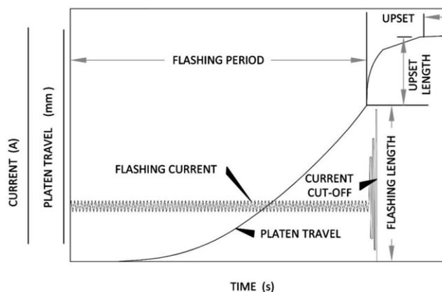
Fig. 1 : Schematic of flash butt welding process
