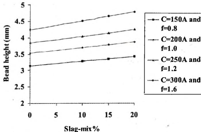
**Fig. 2 Direct effect of slag-mix % on bead height**
