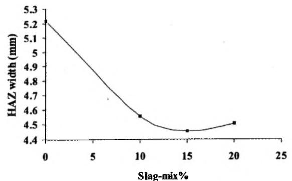
**Fig. 11** Interaction effect between flux basicity index and slag-mix % on HAZ width (C=300A & 0.8 <= f <= 1.6)
