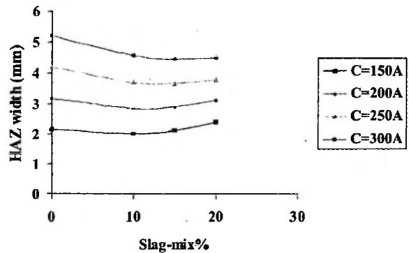
**Fig. 7** Interaction effect between current and slag-mix % on HAZ width (f=1.2)
