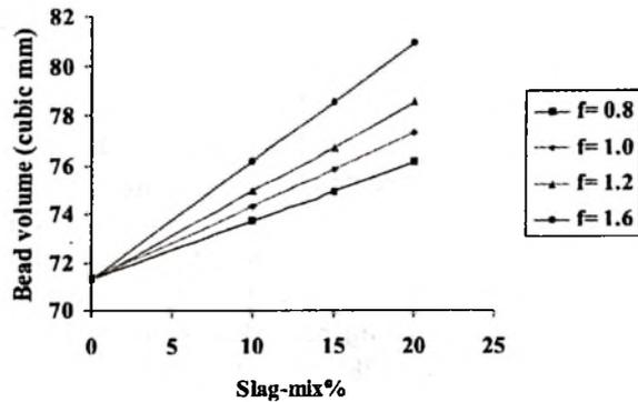
**Fig. 12 Interaction effect between flux basicity index and slag-mix % on bead volume (C=300A)**
