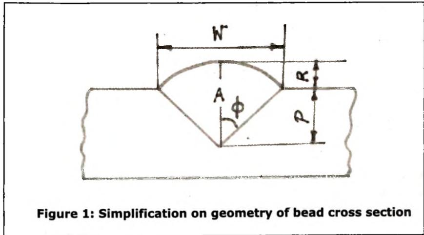
**Figure 1: Simplification on geometry of bead cross section**
