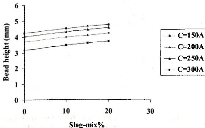
**Fig. 5 Interaction effect between current and slag-mix % on bead height (f=1.6)**
