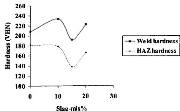
**Fig. 15: Effect of slag-mix% on hardness of weldment and HAZ (Current= 150A and f= 1.6)**
