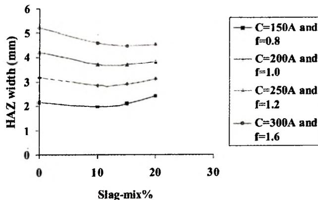
**Fig. 3 Direct effect of slag-mix % on HAZ width**
