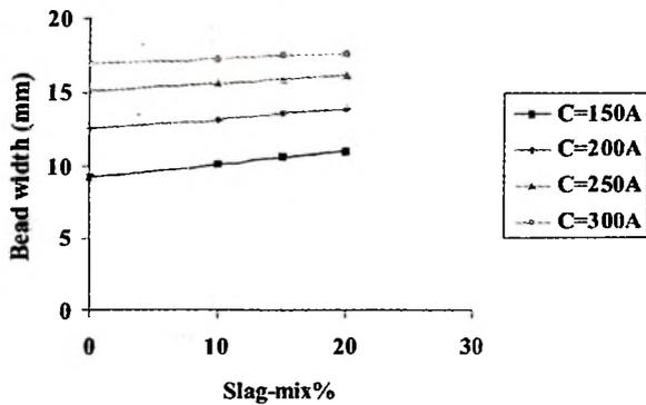
**Fig. 6** Interaction effect between current and slag-mix % on bead width (f=1.6)
