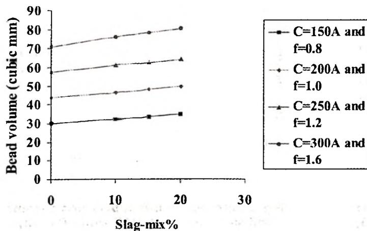
**Fig. 4 Direct effect of slag-mix % on bead volume**
