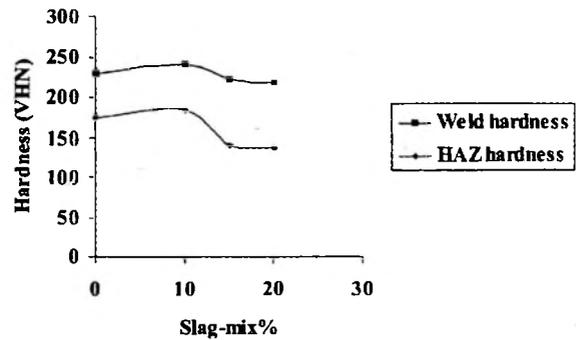
**Fig. 13: Effect of slag-mix% on hardness of weldment and HAZ (Current= 150A and f= 0.8)**
