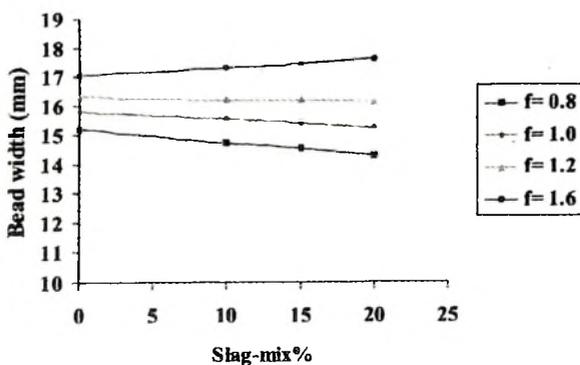
**Fig. 10** Interaction effect between flux basicity index and slag-mix % on bead width (C=300A)
