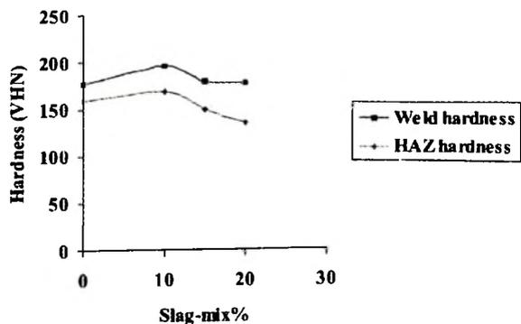
**Fig. 14: Effect of slag-mix% on hardness of weldment and HAZ (Current= 300A and f= 0.8)**
