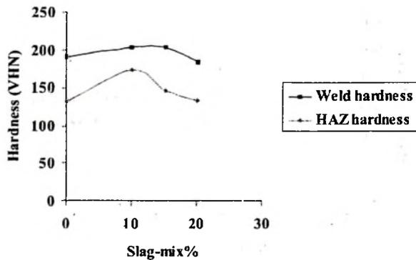
**Fig. 16: Effect of slag-mix% on hardness of weldment and HAZ (Current= 300A and f= 1.6)**
