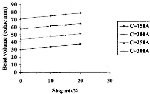
**Fig. 8** Interaction effect between current and slag-mix % on bead volume (f=1.2)
