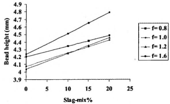
**Fig. 9** Interaction effect between flux basicity index and slag-mix % on bead height (C=300A)
