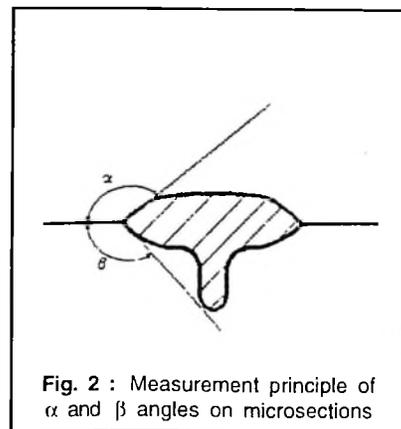
**Fig. 2 : Measurement principle of  $\alpha$  and  $\beta$  angles on microsections**
