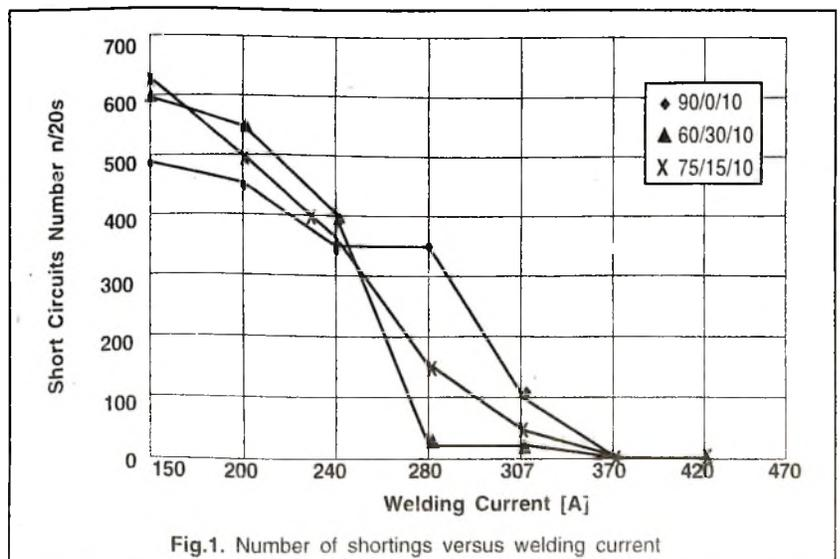
Fig.1. Number of shortings versus welding current
