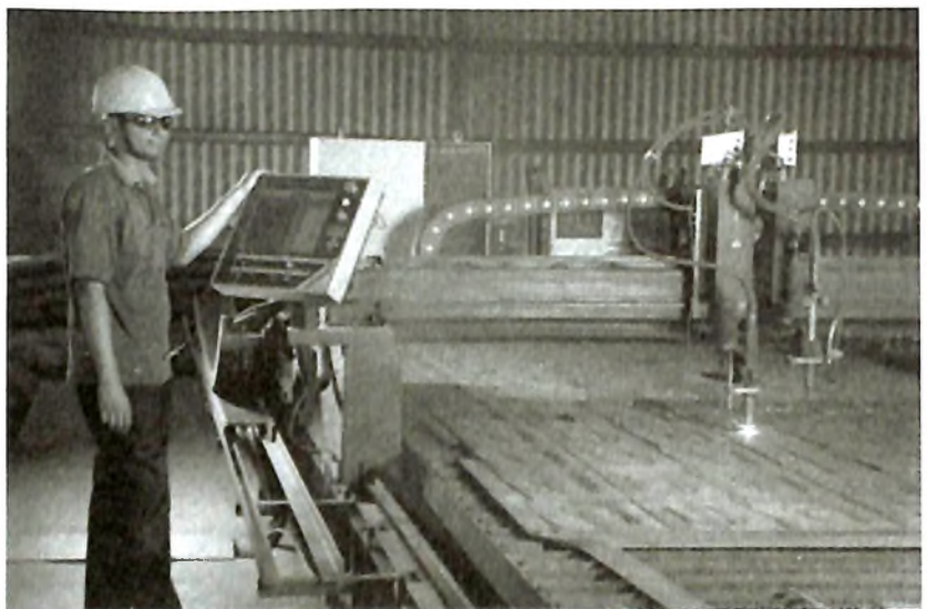
CNC Plasma cutting of profiles
