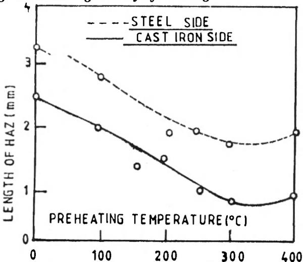
Fig. 2. : Effect of preheating temperature of work piece material on the corresponding 'HAZ'.
