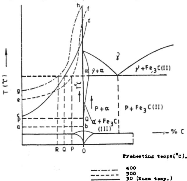
Fig. 3. : Effect of preheating the work piece material on the corresponding temperature distribution model diagram during welding.
