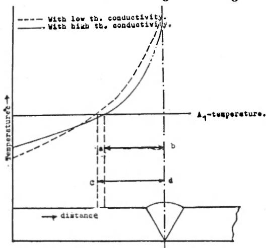
Fig. 4. : Temperature distribution model diagram for work piece material with varying thermal conductivity. (ab = HAZ when thermal conductivity is high, cd = HAZ when thermal conductivity is low.)
