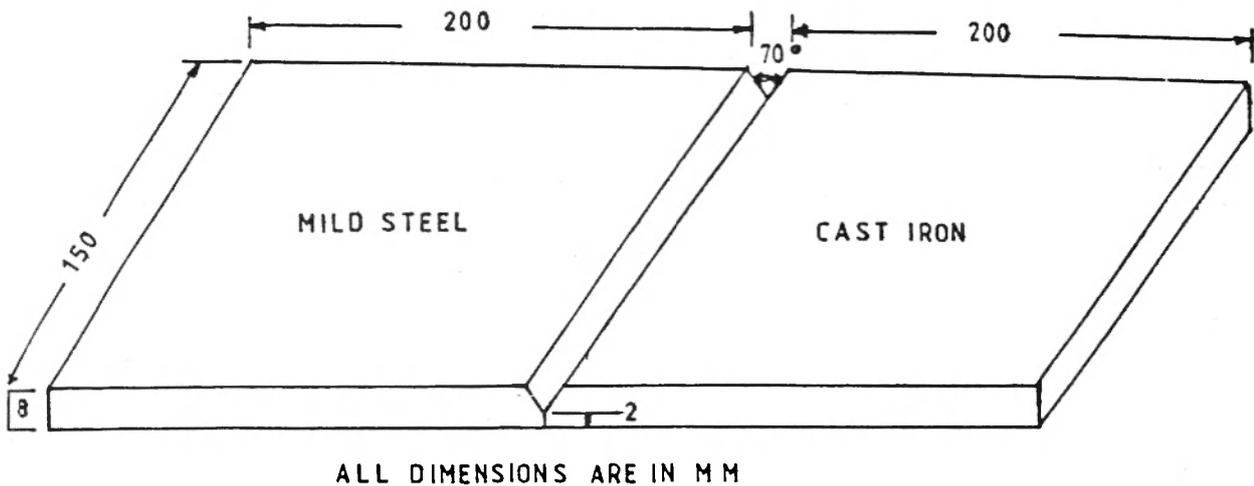
Fig. 1. : Groove geometry of Welding
