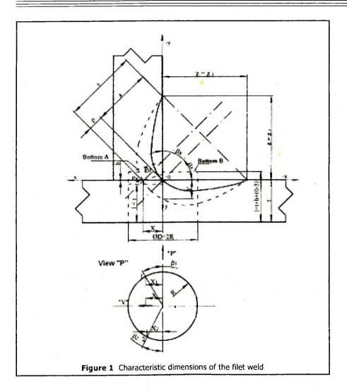
estimating the carrier dimension of the fillet. As the carrier dimension the non-obligatory value "a" is needed to be used.
