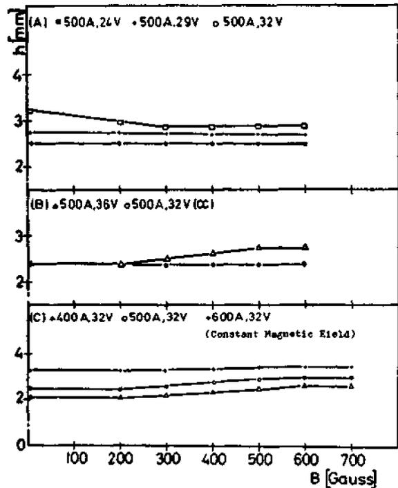
Fig. 7. Effect of magnetic flux density  $B$  on weld reinforcement  $h$ .
