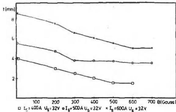
Fig. 9. Effect of magnetic flux density  $B$  on weld penetration  $t$ , (constant magnetic field).
