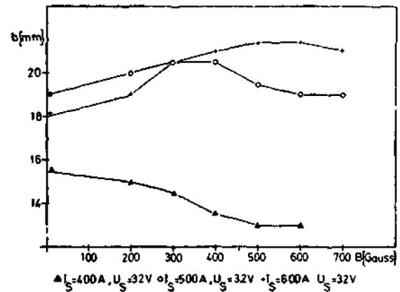
Fig. 8. Effect of magnetic flux density  $B$  on weld width  $b$  (constant magnetic field).
