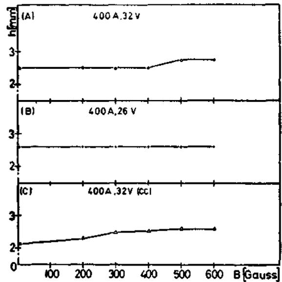
Fig. 6. Effect of magnetic flux density  $B$  on weld reinforcement  $h$ .
