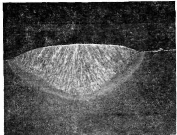
Fig. 11. Weld cross-section at : 625A, 36V, 75cm/min and 400 G.
