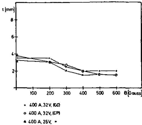
Fig. 4. Effect of magnetic flux density  $B$  on weld penetration  $t$ .
