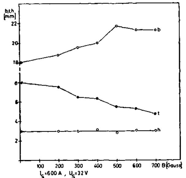
Fig. 3. Effect of magnetic flux density  $B$  on weld width  $b$  penetration  $t$ , and reinforcement  $h$ .
