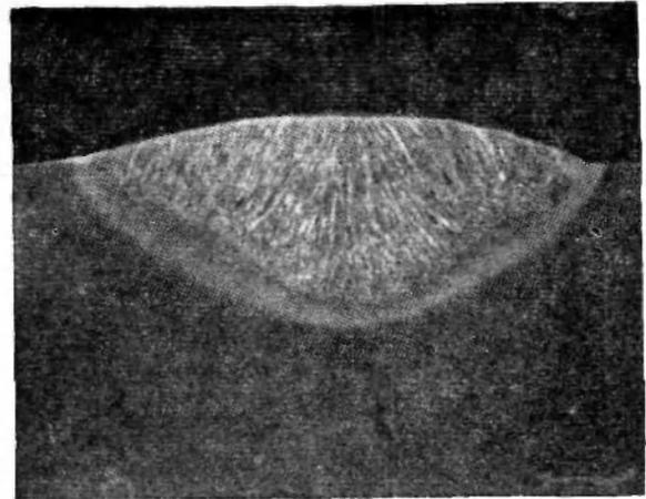
Fig. 10. Weld cross-section at : 500A, 32V, 40cm/min and 0 G.
